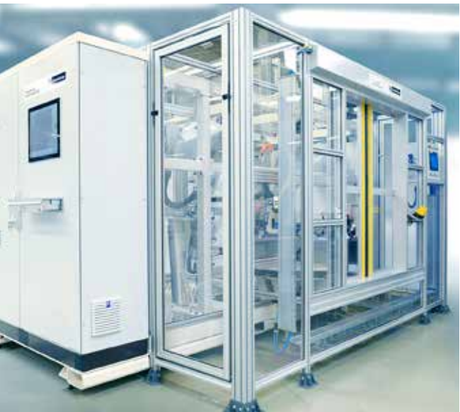
Example of an End of Line Test bench for turbochargers
