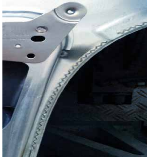
Sinusoidal seam on a part
