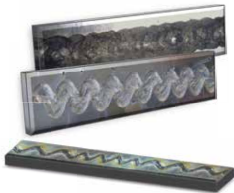
Sinusoidal seam by use of scan unit
