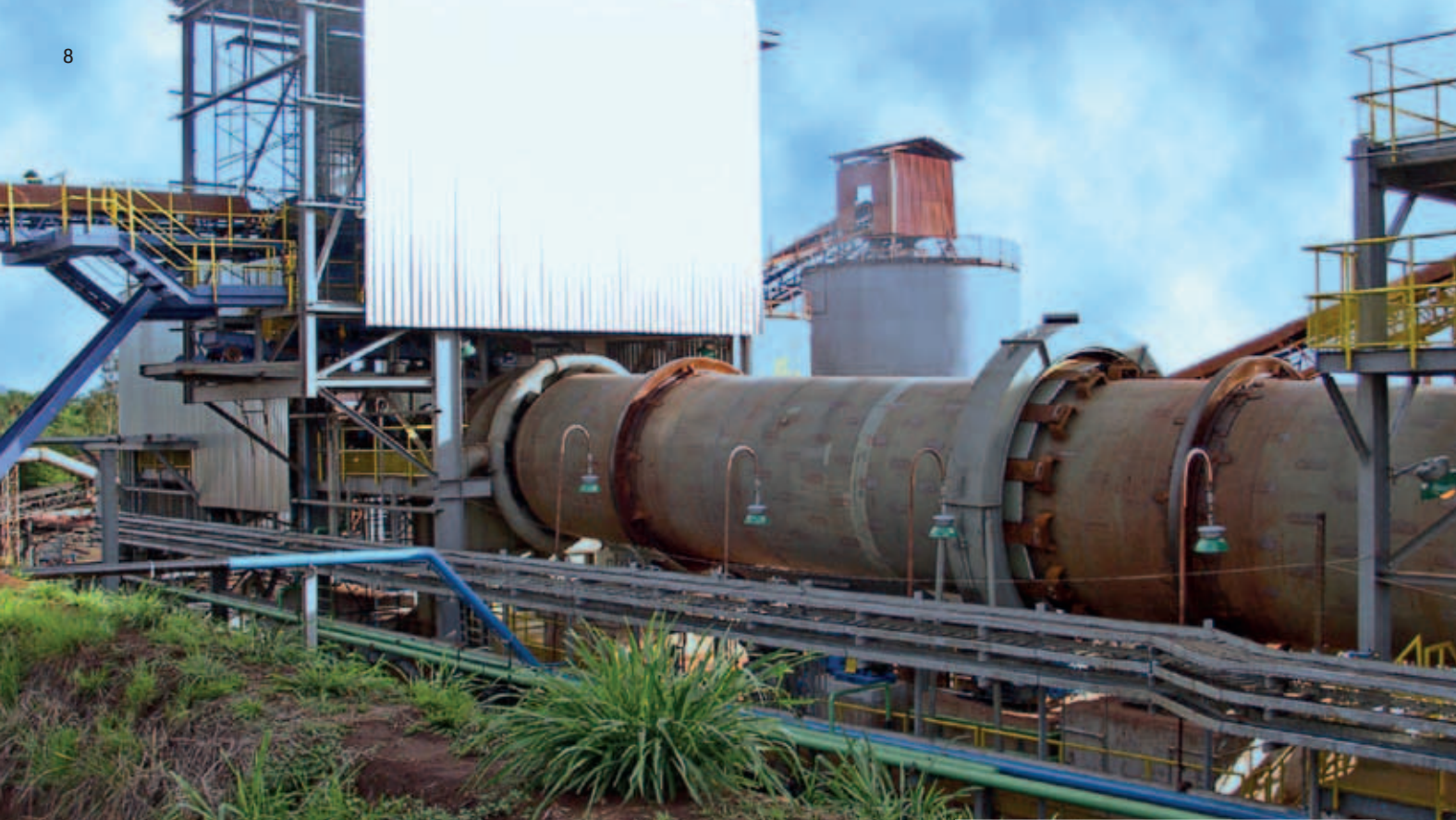
Rotary dryer for nickel ore in Brazil.
