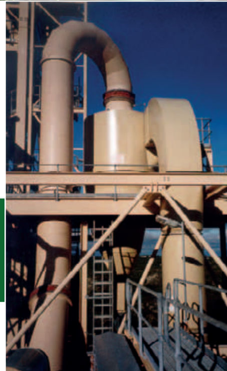
Shaft-type flash dryer in a lime production plant in Australia.
