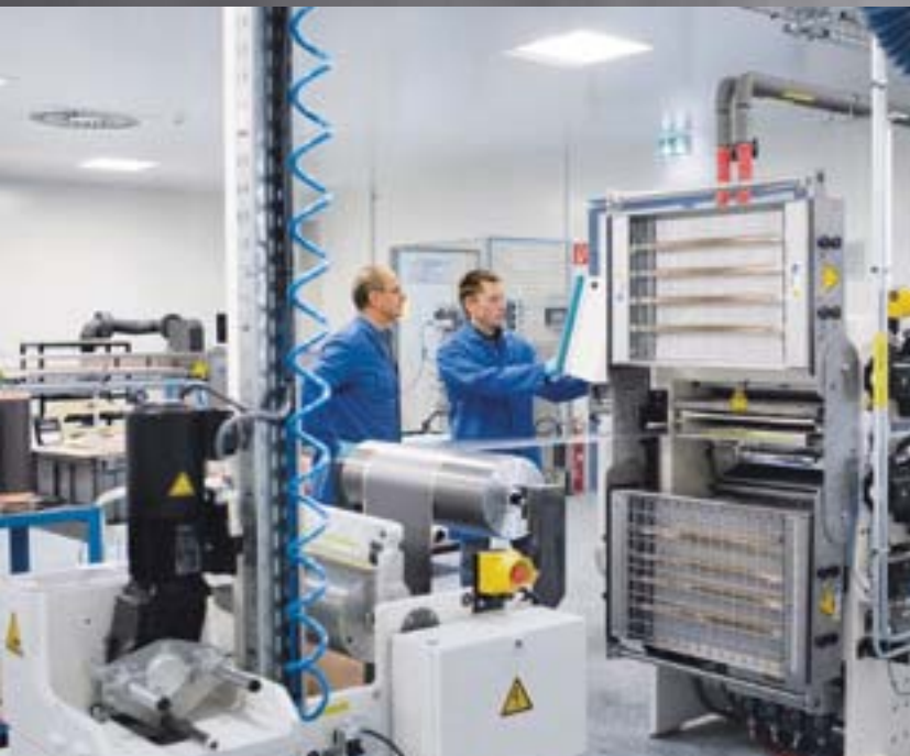
Under pressure: A calender machine compresses the battery electrodes – a key step in the production of a battery system.
