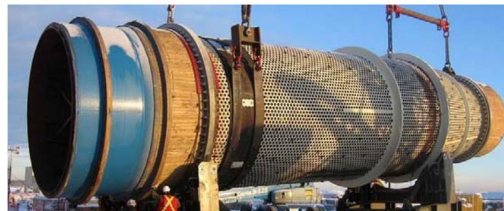
Rotary breaker for oil sand mining
