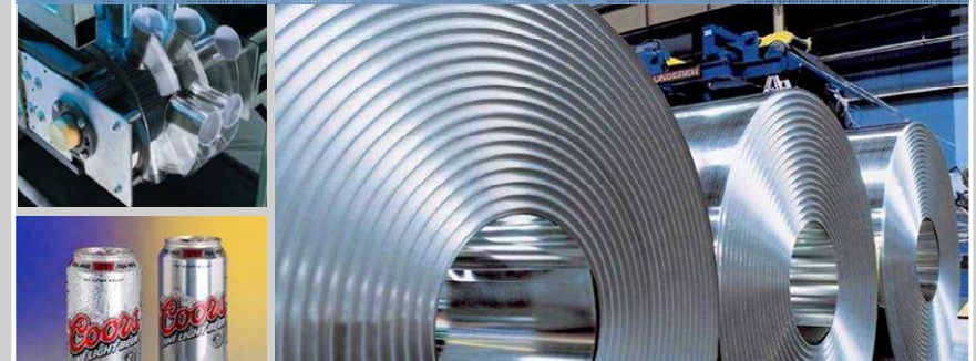
Can wall thicknesses of 0.07 mm place extreme demands on deep drawing properties
