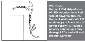
6. Connections: Modules may be connected in series or parallel.
