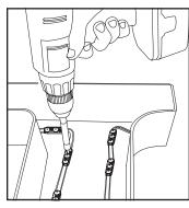
Fasteners: If desired, modules can be secured with #6 (3.5 mm) pan head sheet metal screws or ½ in (3 mm) aluminum rivets.
