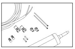
2. **Supplies required:** PLTC cable, wire nuts, IDC connectors or butt splices with appropriate safety agency markings, and cable ties. <u>Optional</u>: Screws and silicone.
