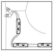
Cap all unused wires: The strand of modules should not be looped to create a closed circuit.
