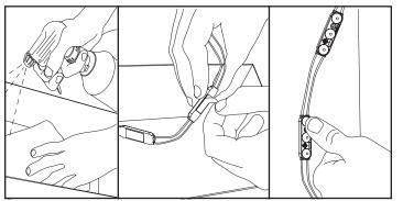
4. **Peel and stick:** Clean inside sign with rubbing alcohol and allow to dry. Using predetermined layout and LED placement from Step 3, remove tape backing and stick modules into place. Ensure modules are firmly attached.
