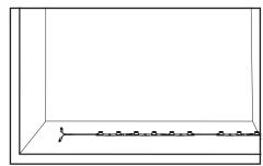
2a. Secure modules to sides of sign box using #8 (M4) pan head sheet metal screws or 5/32" (4 mm) aluminum rivets.
