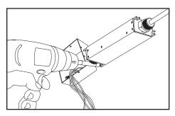
**5.** Units may be mounted in any orientation using mounting tabs.
