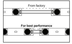
**TIP:** For best results, space Long modules 2/m (19.7" on center) and Short modules 4/m (9.8" on center). For best performance in a single-sided box, mount modules on returns, near rear wall of box ( $\sim$ .5 – .75" [1 – 2 cm]). For a double-sided sign box, mount modules in center of returns.
