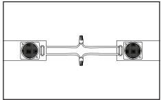
Connections: Modules may be connected in series or parallel. Modules should not be looped to create a closed circuit. Cap all unused, exposed wire ends.
