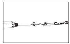
Connect to power supply: Using UL Listed electrical connectors, daisy chain product as required and connect to power supply.
