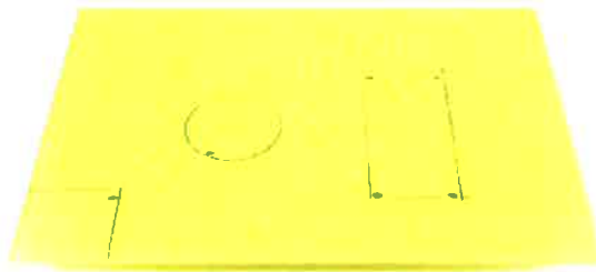
Fig. 1 The ideal sheet size For use indoors, at least 3 mm must be allowed per meter of length and width. This should be considered when ordering the sheets.
