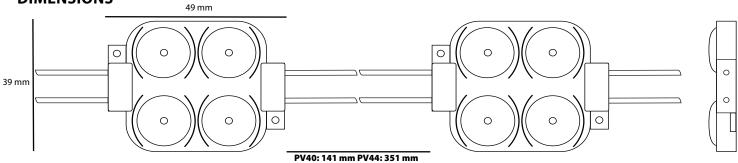
PV40: 190 mm PV44: 400 mm at maximal cable length
