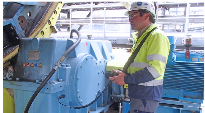
Vibration measurements on a spur gear unit
