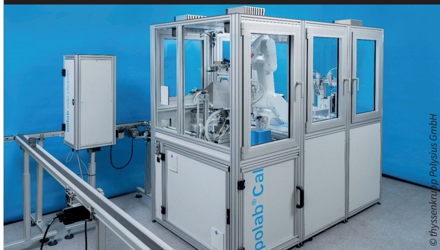
Figure 2: polabCal with temperature-controlled housing, connected to automated sampling system at customer site
