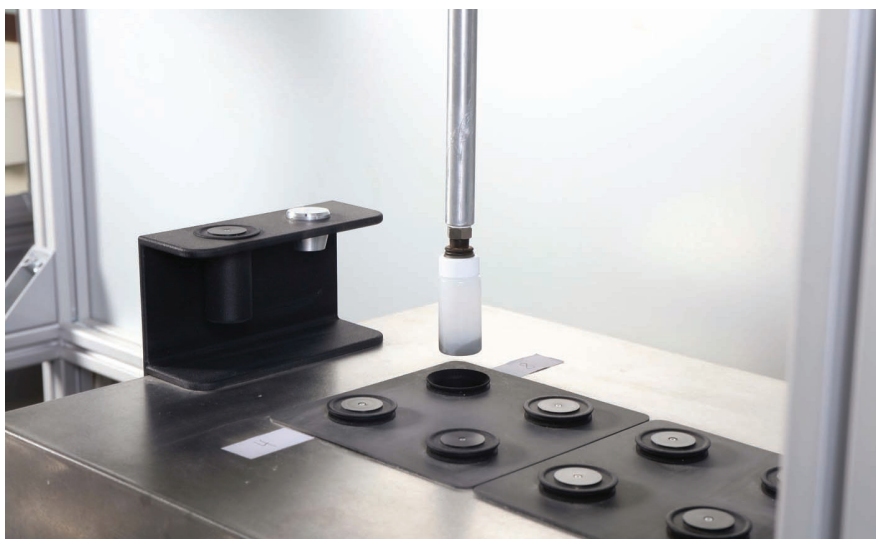
Figure 3: I-Cal Flex calorimeter in automated operation. Each cell is operated by polabcal and can be exchanged individually for maintenance
