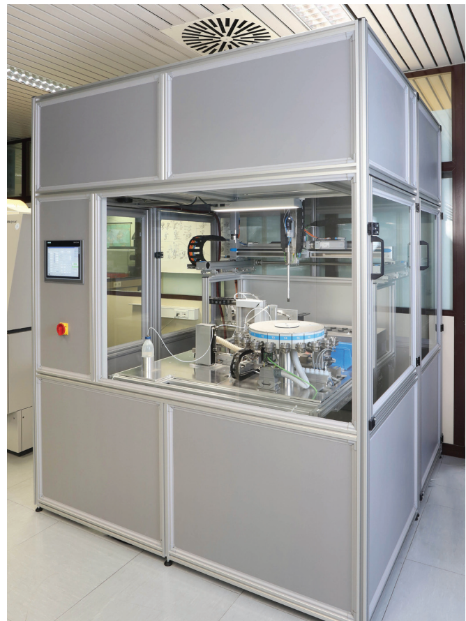
Figure 1: polabcal – the first automated calorimeter (with air-conditioned housing and PLC controller)
