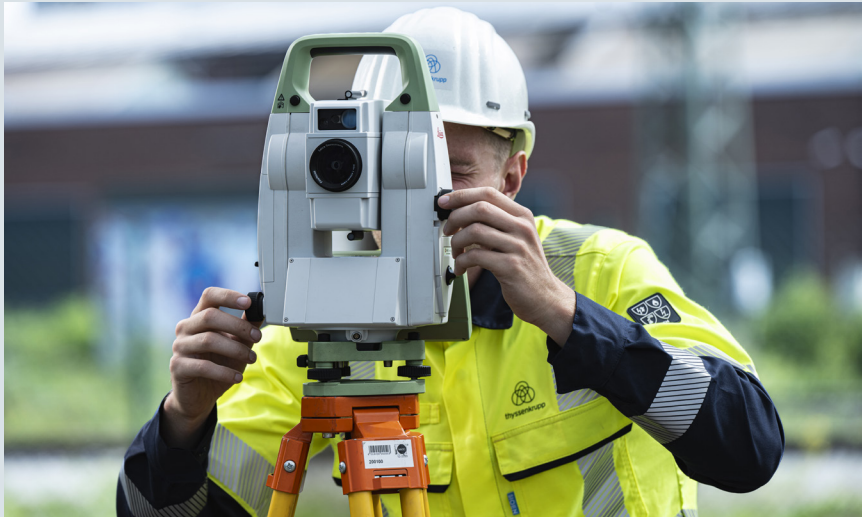
polscan® - High-precision optoelectronic measuring system at on-site use.
