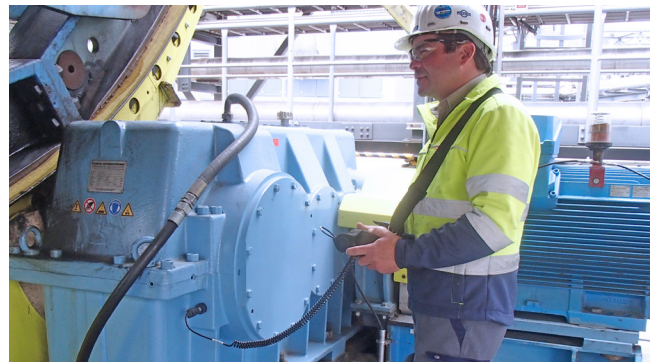
Vibration measurements on a spur gear unit
