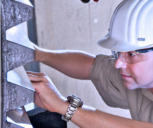
Checking the "static contact pattern" of large tooth gearing
