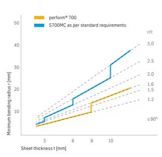
perform® 700 is significantly better suited to bending and press braking than to the comparative grade according to EN 10149-2.
