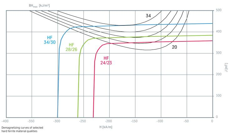
a = anisotropic; i = isotropic The magnetizing field strength is at least three times the  $\rm H_{cJ}$  value. The relative permeability ( $\mu_p$ ) is between 1.05–1.10.
