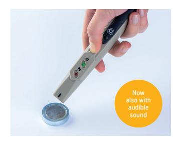
Sensitivity: approx.  $\pm$  15 mT on/off hysteresis Battery: 4 \* 1,5 V button cells LR 44/A 76
