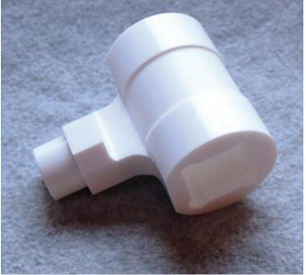
Ertalyte<sup>®</sup> part completed using 5 Axis Machining.
