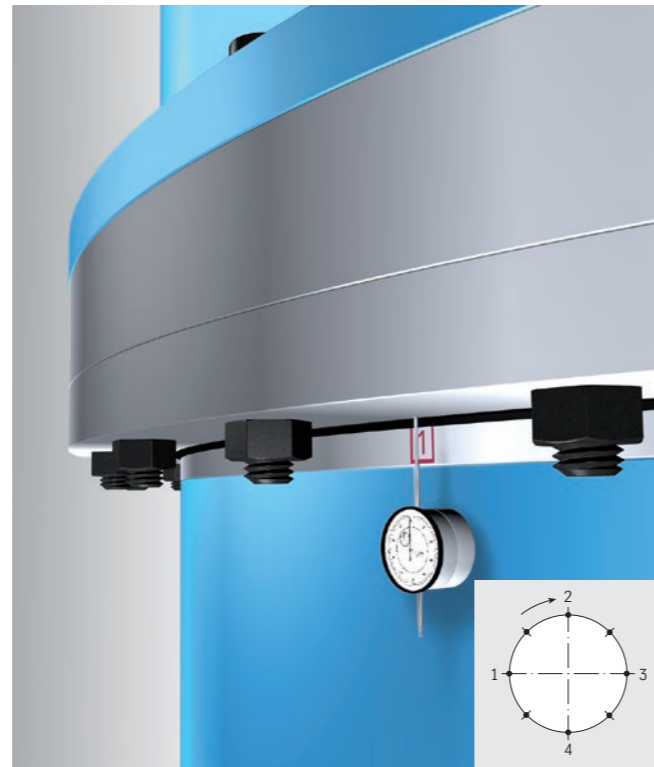
Figure 34: Basic setup for measuring the tilting clearance
