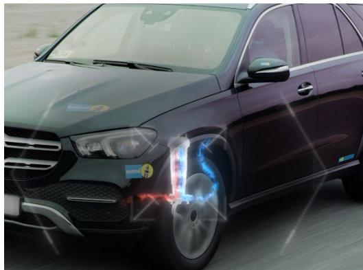
Equipped with the innovative combination of a conventional controlled shock absorber and an active hydraulic cylinder, eSuspension technology enables fully active adjustment of the suspension to any driving situation - for an unprecedented feeling of comfort in any driving situation.
