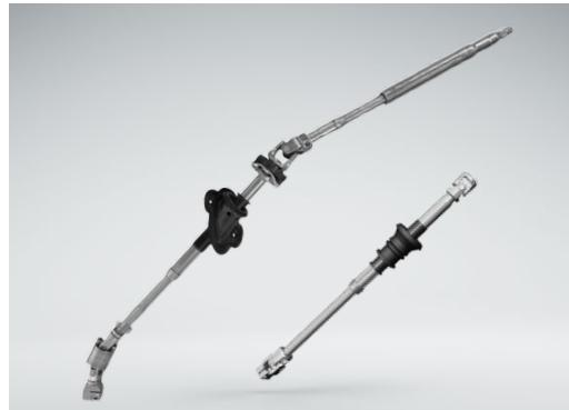
Spindles and I-Shafts are the base for the internal axis of the column. They transfer torque from the steering wheel to the steering gears. Their main tasks are ensuring length compensation, crash functionality & steering feel.
