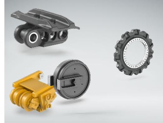
Complete range of undercarriage components for crawler machines (bulldozers, excavators, others) across all market segments (mining, construction, forestry).
